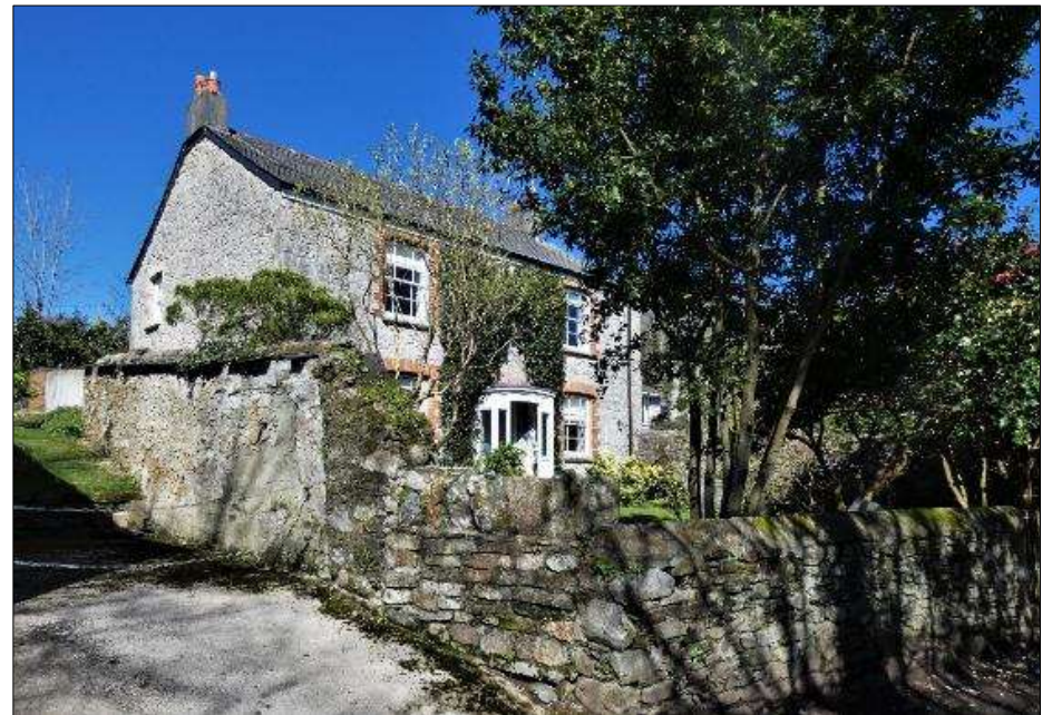
House with moorstone and killas wall to the front and an unusual survival of a cob wall with slate coping to the side.
